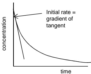
In the experiment between sodium thiosulphate and hydrochloric acid we usually measure reaction rate as **1/time** where the time is the time taken for a cross placed underneath the reaction mixture to disappear due to the cloudiness of the Sulphur.  $\text{Na}_2\text{S}_2\text{O}_3 + 2\text{HCl} \rightarrow 2\text{NaCl} + \text{SO}_2 + \text{S} + \text{H}_2\text{O}$
