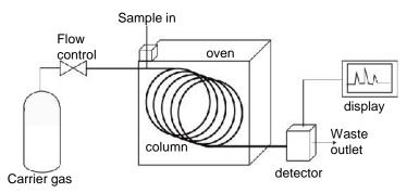
It is important to use an inert carrier gas such as helium or nitrogen. These will not react with the components being separated in the GC column.
