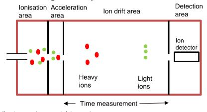
The mass spectrometer can be used to determine all the isotopes present in a sample of an element and to therefore identify elements.
