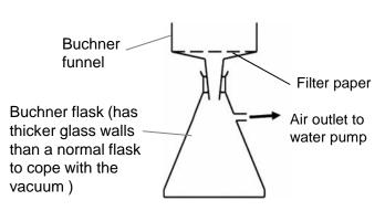
This is vacuum filtration. The apparatus is connected to a water pump which will produce a vacuum. Use if larger amounts of solid are formed.
