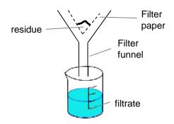
This is gravitational filtration. Use if small amounts of solid are formed.
