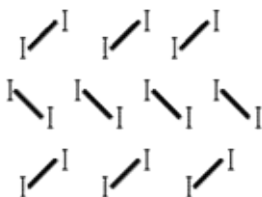
Regular arrangement of \text{I}_2 molecules held together by weak van der Waals forces
