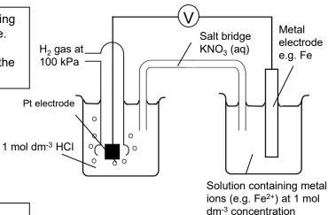
Because the equilibrium does not include a conducting metal surface, a platinum wire is used which is coated in finely divided platinum. (The platinum black is used because it is porous and can absorb the hydrogen gas.)
