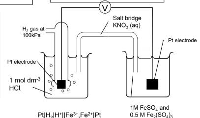
Note: in the electrode system containing two solutions it is necessary to use a platinum electrode and **both** ion solutions must be of a 1 mol dm<sup>-3</sup> concentration, so  $[Fe^{2+}] = 1$  mol dm<sup>-3</sup> and  $[Fe^{3+}] = 1$  mol dm<sup>-3</sup>.
