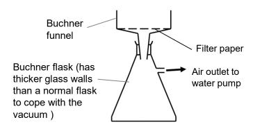
This is vacuum filtration. The apparatus is connected to a water pump which will produce a vacuum. Use if larger amounts of solid are formed.
