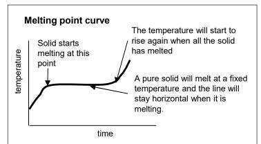
The temperature does not rise when the solid is melting because the heat is absorbed to break the bonds between the solid particles
